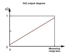
To ensure a good linearity, wire the potentiometer as a voltage divider and never as a rheostat. The input resistance of the operating system must be very high (greater than  $10M\Omega$ )
